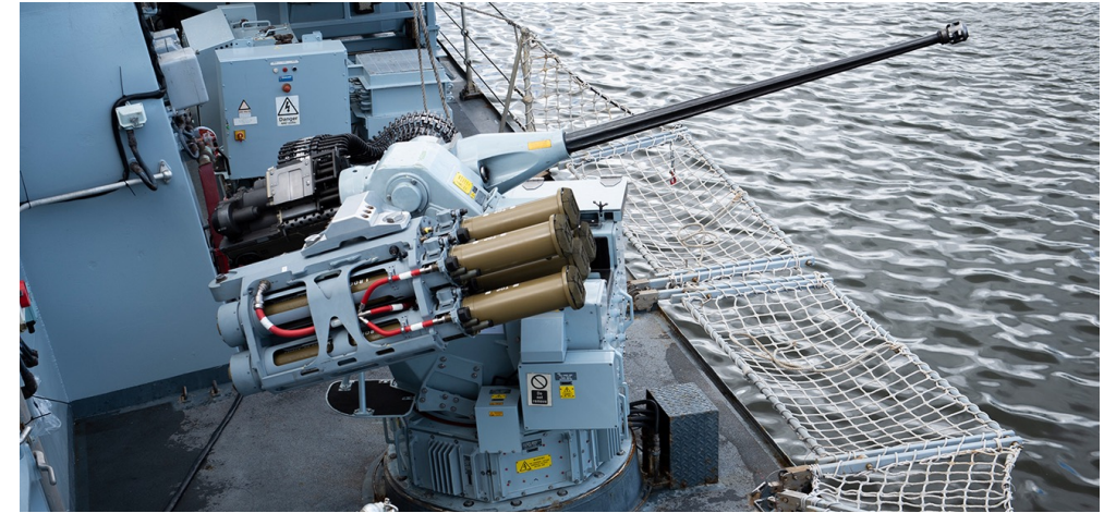
Image: A sample Hybrid Gun Missile System, known as SIGMA, which combines two combat proven systems; The DS30 automated gun from MSI UK and the Lightweight Multirole Missile from Thales UK on a single mount.
